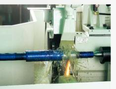
Wheel forming device (For NC model, with auto compensation) (Optional) The device functions as the manual wheel forming device. It further employs an automatic hydraulic unit, and compensation parameters are able to be set during operation (driven by motor) for fast grinding compensation.
