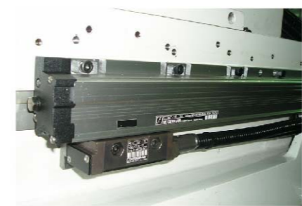
Linear Scale For Z Axis (Optional) • The linear scale provides closed-loop control, assuring extremely high positioning accuracy and stability.
