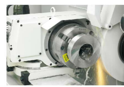
Plunge Cylindrical Grinding • Two axes control combined with one auxiliary axis for workhead spindle running. • Least input increment: 0.001 mm.
